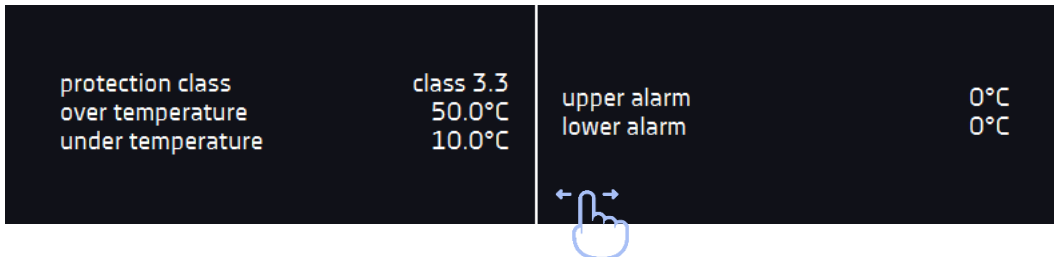
Figure 12 - Status – protection and alarms
